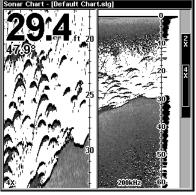
Split Zoom Sonar Chart. Left, image shows the left window zoomed to 2X. The image on the right shows the left window zoomed to 4X. The depth overlay data is set to the default large text size; the water temperature is set to the small text size.
